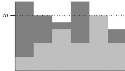
Fig. 3. Light gray area  $la$  represents the number of cars out over time. The  $m$  line shows the pool size for any of the first three methods. Utilization is computed as  $la/(\text{area of } m \text{ rectangle})$ . The dark gray area  $da$  represents the changing TCP pool size. TCP utilization is computed as  $la/da$ .
