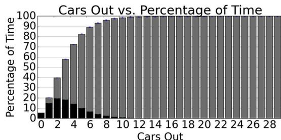
Fig. 4. Black distribution shows the probability of a specific number of vehicles being out of the pool. The gray distribution shows the cumulative distribution function.
